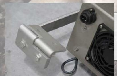
We've designed a swing hinge that allows the unit to be swung out of the way when work is needed on the beds. The hinge is also a pop-off design which allows service to be easily completed by
